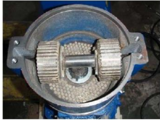
6.2.1 Open the upper case, the take out the roller.
